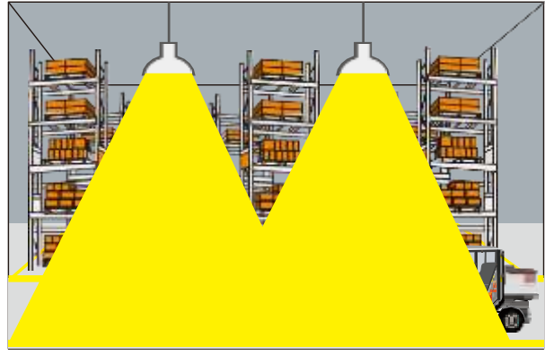
With insufficient ambient light, the lamp switches on when motion is detected.
