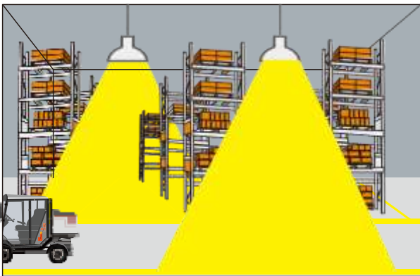
After hold time, the lamp dims to a low light level if no new motion trigger.
